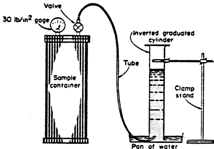
U.S. Bureau of Mines equipment for direct method desorption of coal samples (after Diamond and Levine, 1981, p. 6).
