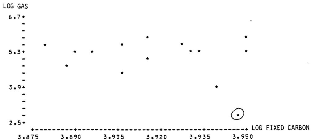
Log-log plots show that if ash, volatile matter, and fixed carbon are similar (given similar thicknesses and depths greater than 1000 feet) gas contents only vary within a relatively narrow range. Circled outlier is from a very thin (1.6 foot) bed.
